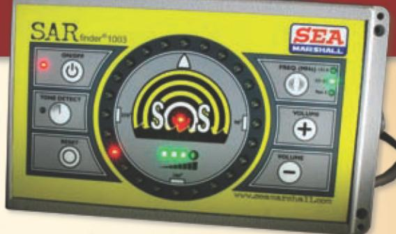
A red LED on the Sea Marshall display indicates the location of the 121.5-MHz alert signal relative to the boat's heading.
