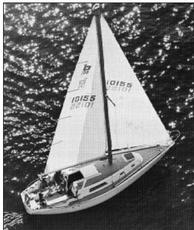
*Contrasting deck colors go a long way towards relieving glare. Note the long tiller, which obstructs the cockpit: here, the helmsman is actually sitting at the front edge of the cockpit.*
