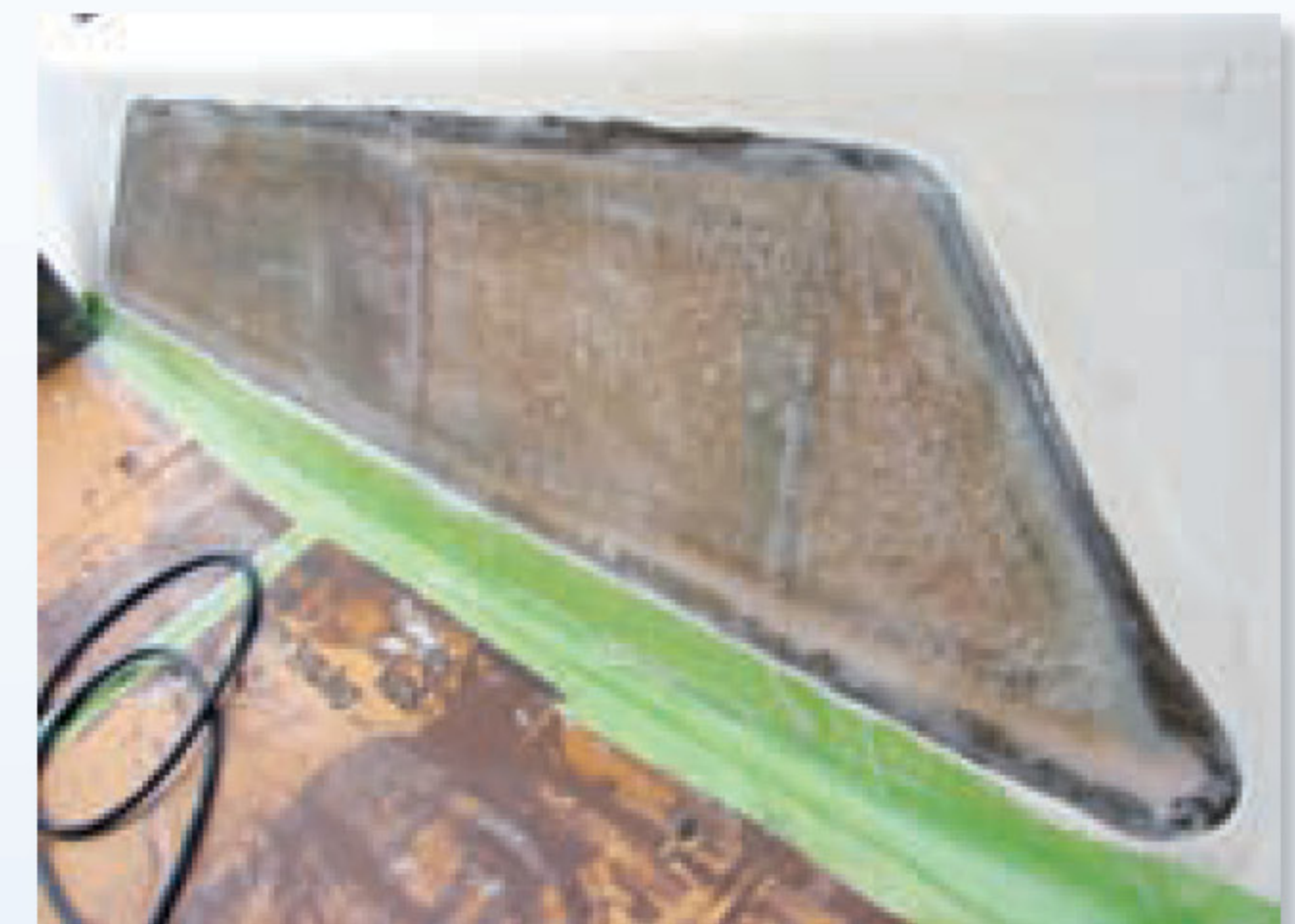
O'Rourke Boat Repair helped reader Bob Davie solve a leaky port problem on his Starflight 38. They glassed in the cut-outs for the original Lexan windows (bottom photos) and installed Lewmar ports (top photo).
