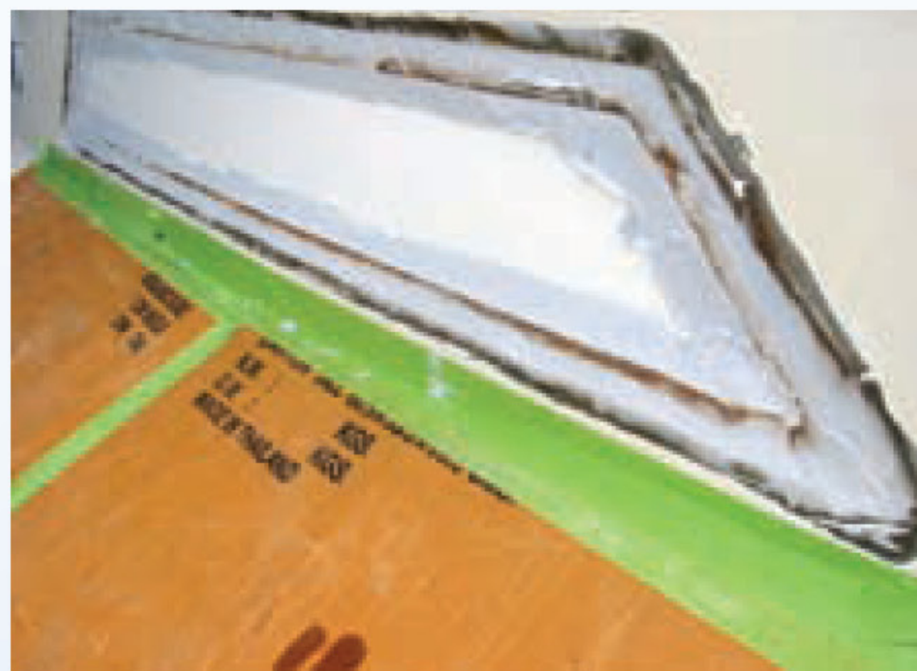
O'Rourke Boat Repair helped reader Bob Davie solve a leaky port problem on his Starflight 38. They glassed in the cut-outs for the original Lexan windows (bottom photos) and installed Lewmar ports (top photo).
