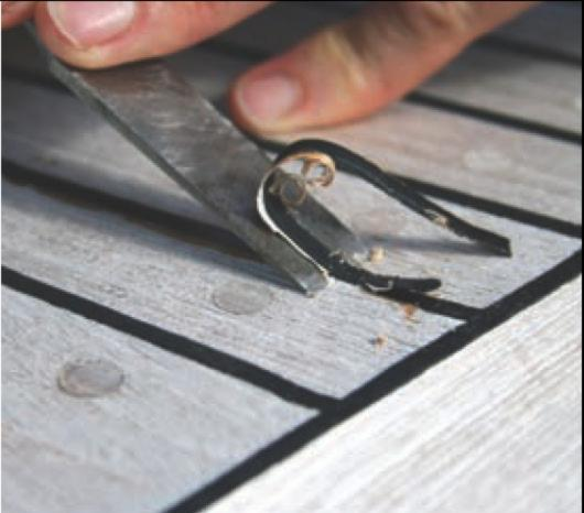
Because salt water is abrasive, it scours the deck as it washes over it, wearing away the softer teak. This, and the constant torture of UV and rain, mean that after a decade or so of sailing, most decks will need to be lightly sanded, and the seams cut back and recaulked.
