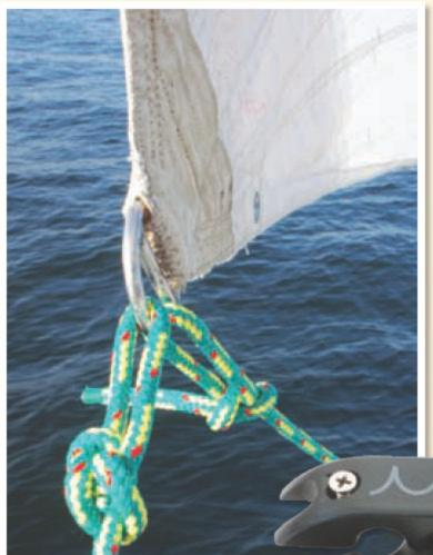
were able to coax the drifter through the gap ahead of the forestay (far left). Furling and resetting the sail on the new jibe also worked well. For sheets, we used New England Ropes Flightline (left), a lightweight Dyneema-core line that floats and sheds water like a duck. Colligo offers a line of two-piece guides (below, left) designed for continuous-line furlers. A furled asymmetrical (below) makes for a compact package to stow.
