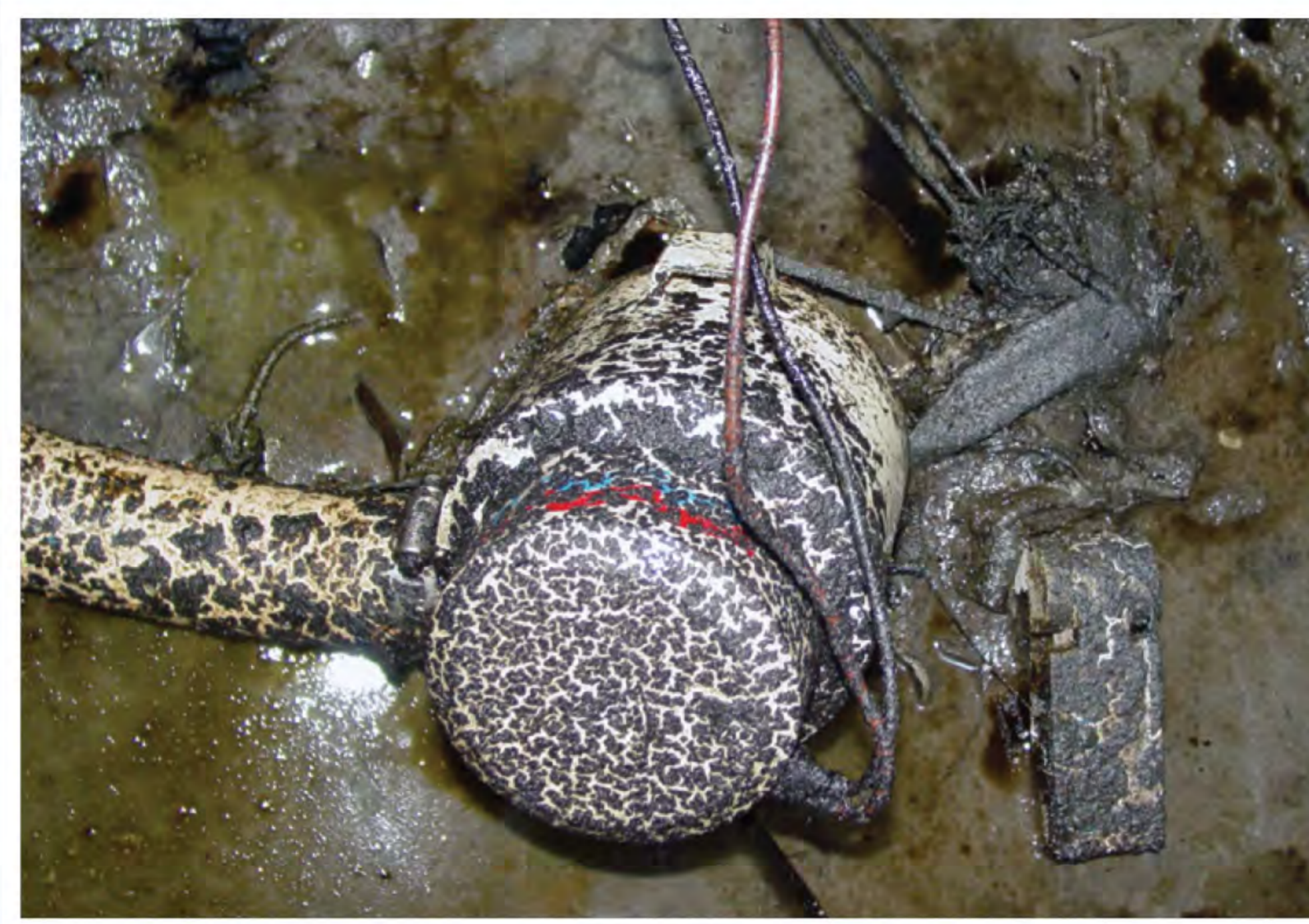
Periodic cleaning will keep your bilge pump from choking under a slurry of ick, unlike this one (above left). Regular inspection of your pump setup should include a look at fittings; notice this pump is missing a hose clamp (above right). .....
