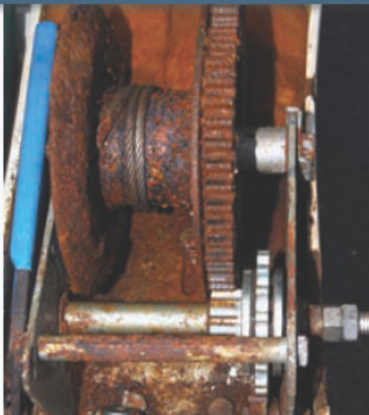
An old trailer winch retrofitted as a swing-keel winch shows its wear.
