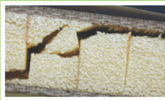
The results of an impact test on a 1-inch-thick cored panel illustrate a classic example of shear failure.
