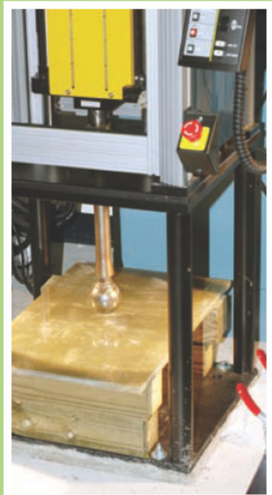
An Instron impact test machine delivers carefully measured point loading on a 3/4-inch solid fiber reinforced polyester (FRP) panel.
