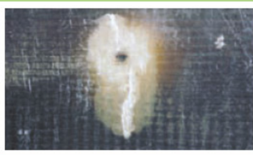
An impact test on a 3/4-inch solid fiberglass panel (shown at right) resulted in this fracture.
