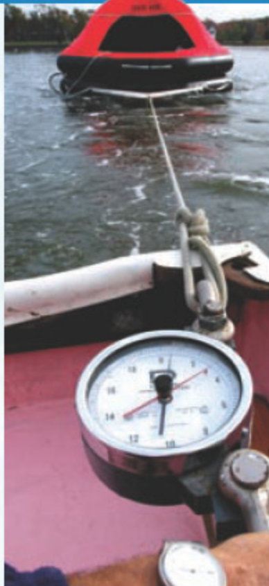
Rafts were towed at 3 knots to evaluate resistance to drift and security of the painter setup.
