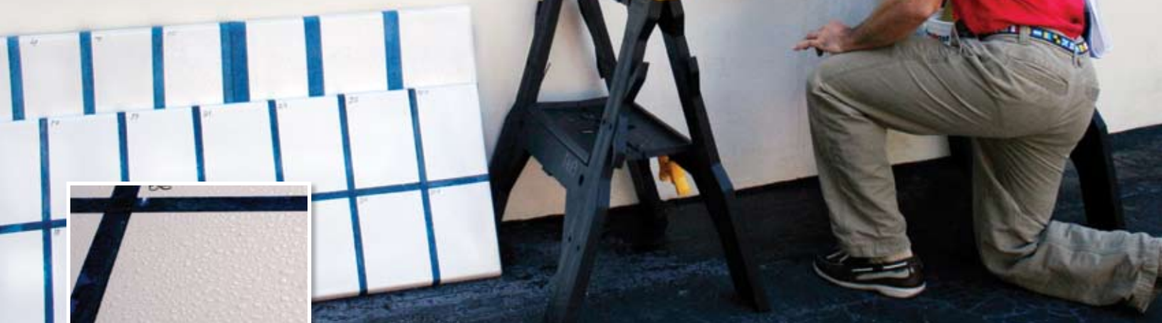
Testers compared each test product's ability to bead water on the fiberglass panels.
