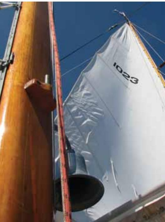
*To get that classic, amber-hued look for a wooden mast or boom, we suggest trying a high-quality flexible spar varnish with UV protection, or trying the route some pros take by applying Awlgrip Awlspar with an Awlgrip Awlbrite overcoat.*
