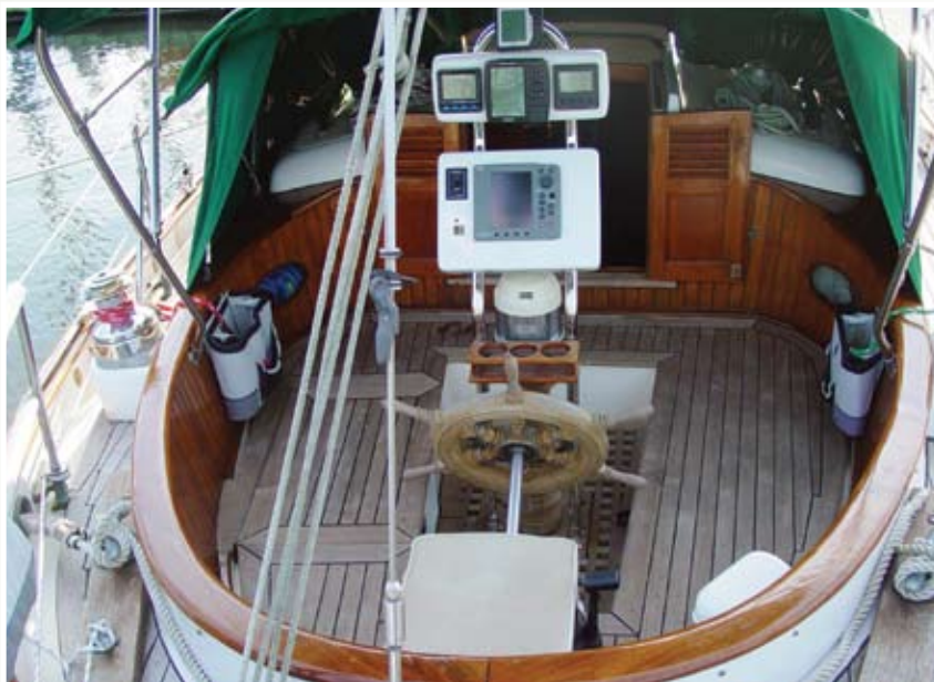
The snug cockpit is ringed in teak. Belaying pins (below, left) are handy for halyard tails. Samson posts (below, middle) offer a fast, easy way to secure anchor snubbers and dock lines. The shallow footwell drains fairly quickly.
