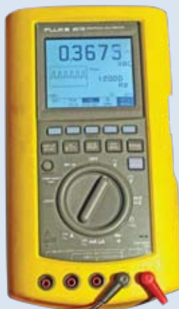
The Tripp Lite MRV2012-UL measured considerable AC ripple leakage during our tests. Excessive ripple can result in a battery overheating.
