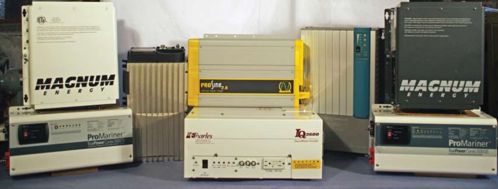
The test field (clockwise from left): Magnum MS2000, Tripp Lite MRV2012, Xantrex Prosine 2.0, Mastervolt Combi, Magnum ME2012, ProMariner Combi 2500QS, Charles IQ-2600, and ProMariner Combi 2000PS.
