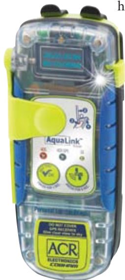
The ACR AquaLink Personal Locator Beacon features a digital readout that gives the user his GPS location. Pushing a dedicated button lets you send an "I'm OK" message to contacts.
