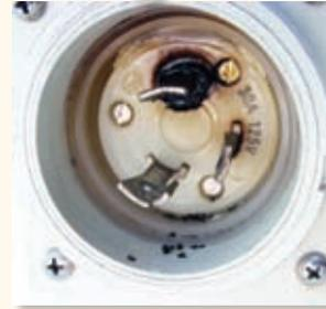
*Once discoloration is visible at the plug face (left) or shoreside socket (right), you'll typically find more damage inside. If left uncorrected, this could create further damage to the system and even lead to a fire.*
