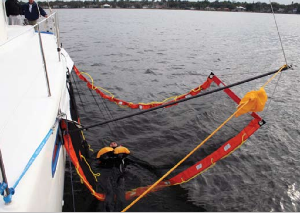
The carbon-fiber pole helps hold the Seascoopa open. Weighted line keeps the leading edge immersed underwater.
