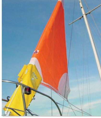
Both the ATN Gail Sail (above, left) and the Storm-Bag from Banner Bay (above, right) are designed to deploy over a furled genoa. We recommend working with a rigger and sailmaker to design a proper hank-on storm jib and stay.
