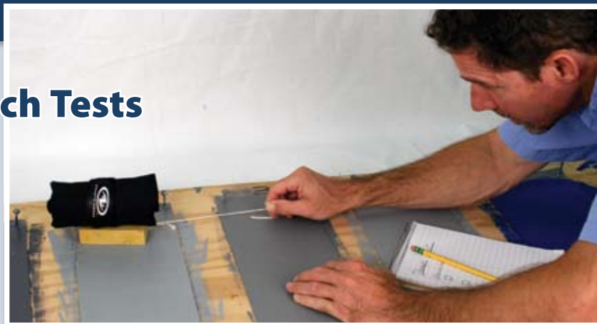
To gauge each coating's abrasion resistance, testers dragged a weighted 320-grit sanding block across each panel three times.
