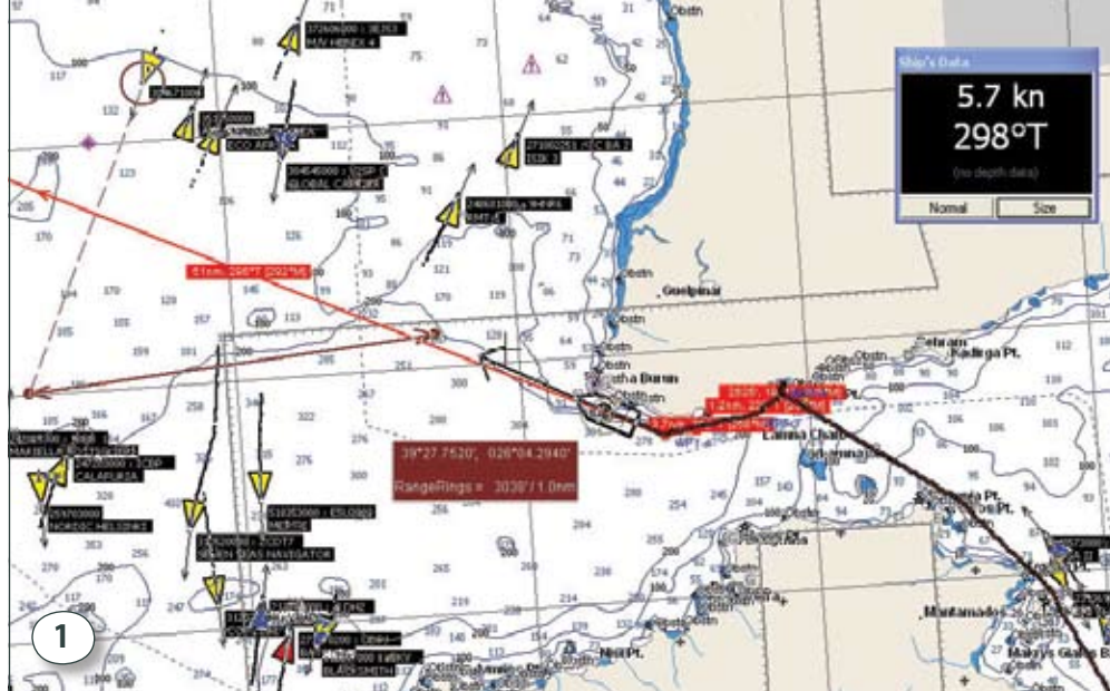
AIS targets clutter Southern Cross' plotter as it starts its passage across the southern approaches to the Dardanelles. The planned route is shown in red, and none of these vessels are in sight yet, but there is already a conflict, shown in red, approaching from the south. Still time to get some planning done.
