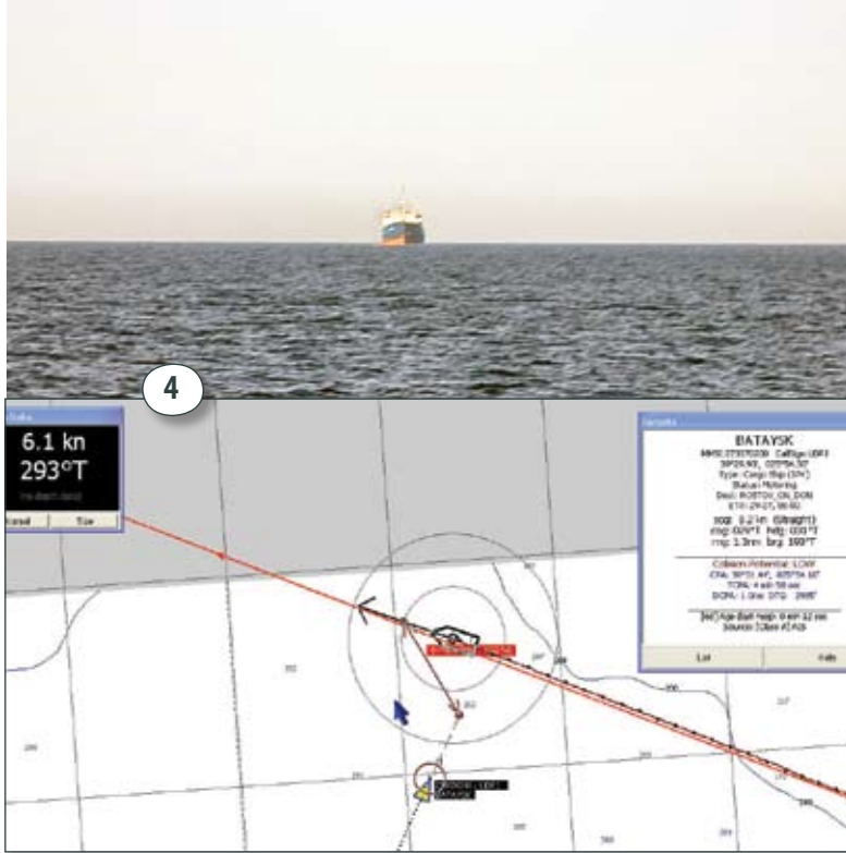
After a few brief moments in the ship's crosshairs, but still keeping a safe distance, they're across. The actual range when they crossed the other vessel's bow was greater than 1.5 nautical miles. They've reduced speed to keep a little in the reserve, which has shortened the predicted CPA to 1 nautical mile, but they are now going safely away from the Bataysk.
