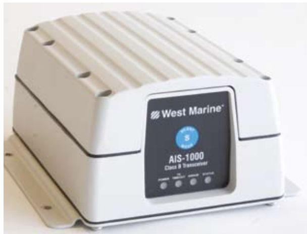
AIS-A transmits more frequent dynamic reports, navigational status, and substantially more static data than AIS-B (above). We tested the AIS-B transceivers from Navico (left) and West Marine (below) for the September 2009 issue.
