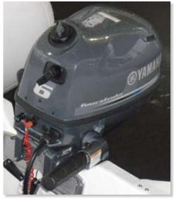
The new Yamaha F4 (above left) and F6 (above) both sport beefy carrying handles on the back of the cowling. The shifters are on the front of the engines.
