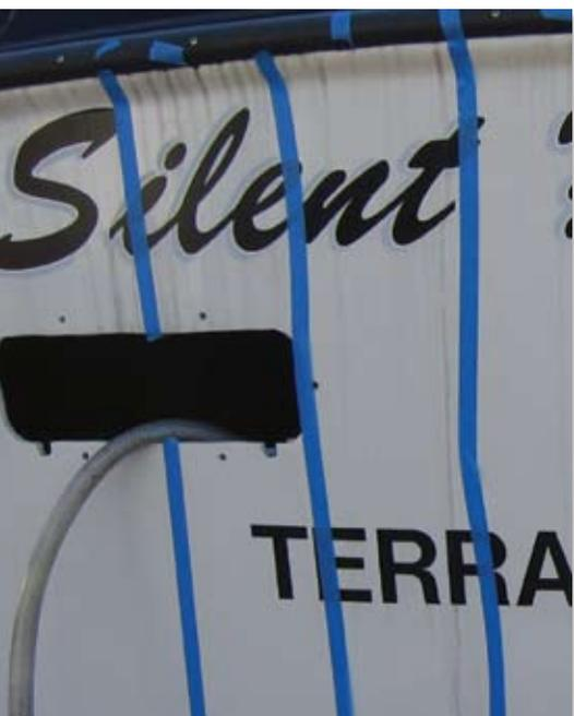
*A blighted Morgan Out Island 41 was the test platform for our 2006 black-streak cleaners test. The streaks develop as polluted rainwater dries on the hull. The best remover we tested was made by Nautical Ease.*
