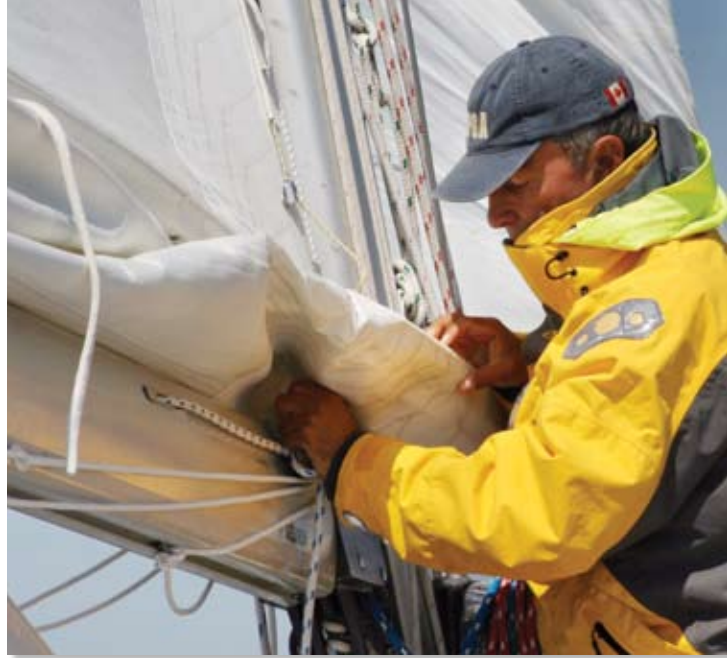
Tack rings for reefing points should be easy to secure on a ram's horn. The reef nettles (or tie points) are tied around the bunt of the sail, not the boom.
