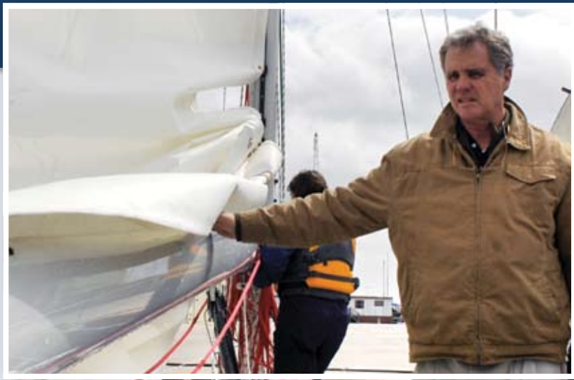
John Jenkins, the head of the Naval Academy's Sail Loft, checks how slides stack and the tack and clew fit the hardware—key areas where problems can arise.
