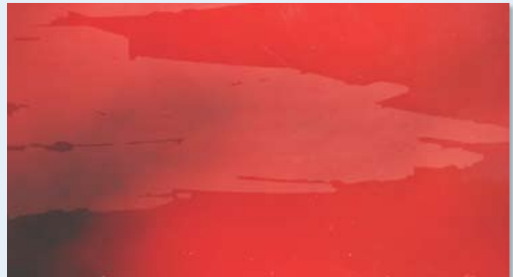
Despite basic pre-painting prep and de-waxing, the LPU lost adhesion shortly after application.
