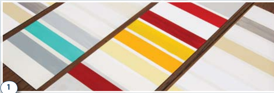
To rate the overall appearance of a paint panel after a year, testers evaluated the coating's color evenness, gloss, and surface texture.
