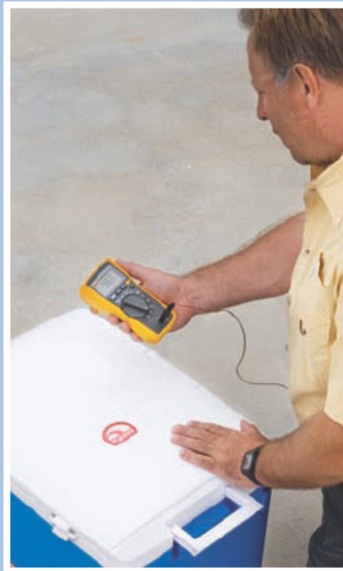
Testers used a temperature sensor, called a thermocouple, to track how well each unit kept its cool over the course of 26 hours.
