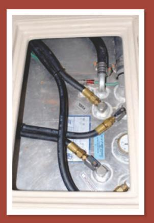
Permanently welded fittings (left, top of photo) limit your options should the welding crack. Black iron tanks (below) are strong and cheap, but prone to corrosion. A deck leak at the fill pipe attacked this tank.
