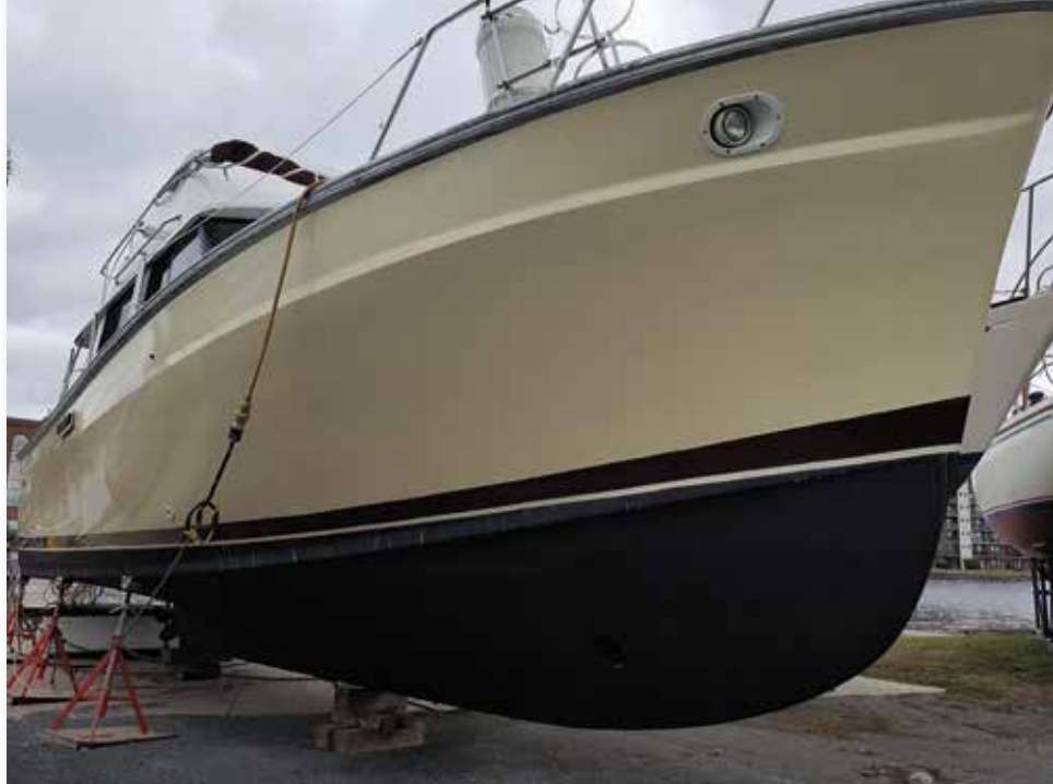
Two liters of Epifanes monourethane yielded three coats on reader Rob Legate's now glossy Mainship. The paint was applied with a close-nap foam roller.
