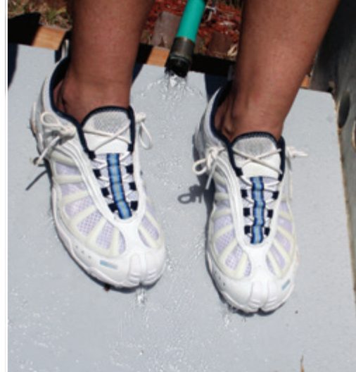
An angled incline was used to evaluate grip both wet and dry. Three successive attempts were averaged for each panel.
