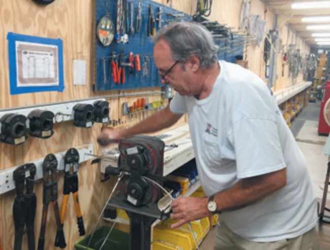
Rigger Glenn Mooney swages a lifeline terminal in his workshop at The Yacht Rigger at Salt Creek Marina, in St. Petersburg, FL.
