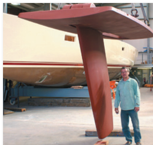
Todd Neville’s Cerulean gleams near its summer home in Mamaroneck on Long Island Sound (above). The boat has a massive, 8,000-pound solid steel swing keel (shown at right with the previous owner at the factory during assembly). The configuration allows it to squeeze into 2 feet, 3 inches of water with the centerboard up. With the centerboard down, it draws nine feet.
