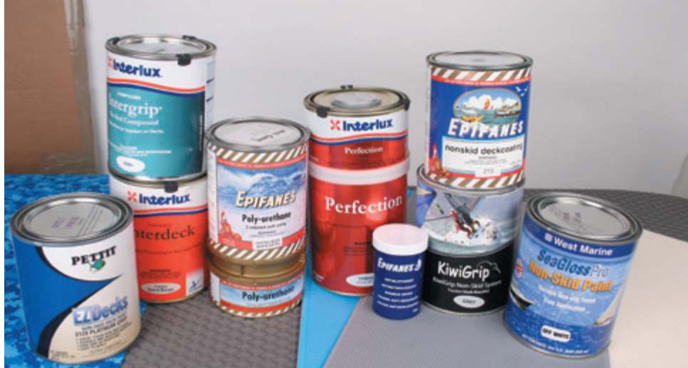
After ten years, finish quality varied by type of paint, with two-part polyurethane paints maintaining their color longer. (West Marine’s paint was discontinued.)
