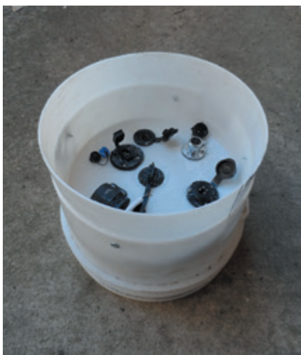
Submerged in our improvised test tank, the Sea-Dog Watertight Connector (inset) proved to be a secure and affordable connector for deck accessories.
