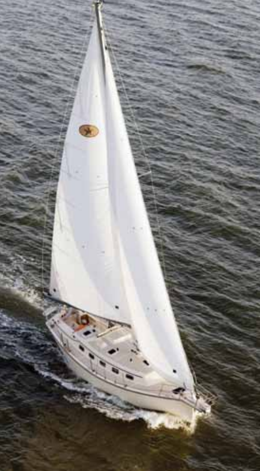
The self-tacking jib on a Hoyt boom emphasizes easy sail-handling.
