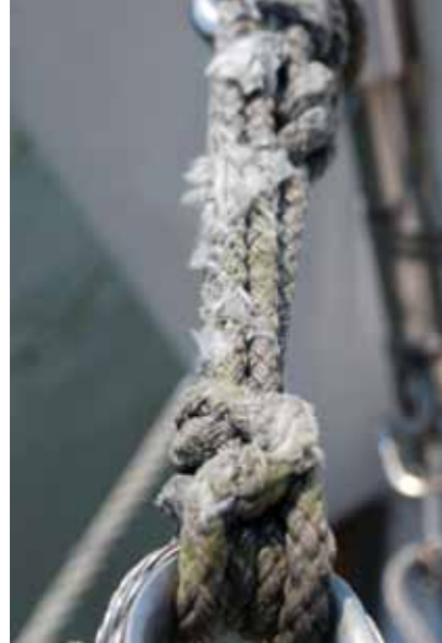
Dyneema lifelines can be lashed to the pulpit (above), rather than relying solely on a welded loop. Abrasion is the biggest foe of fiber lifelines (right). Using lifelines as handholds (below) is a bad habit; a safer practice is using only inboard handholds.
