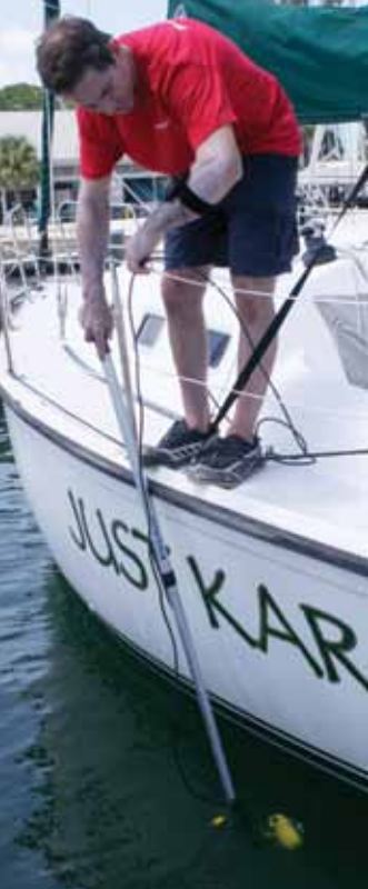
The AquaLens streams real-time video to a small LCD screen worn on the user's forearm.
