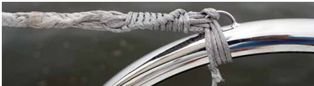
Dyneema lifelines can be lashed to the pulpit (above), rather than relying solely on a welded loop. Abrasion is the biggest foe of fiber lifelines (right). Using lifelines as handholds (below) is a bad habit; a safer practice is using only inboard handholds.
