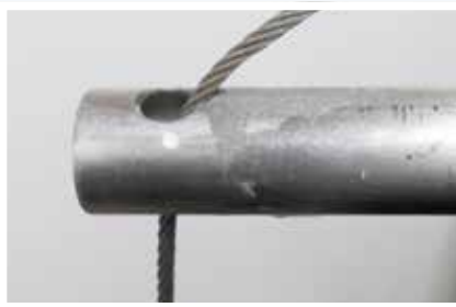
Broken strands were hidden unless the wire lifeline was very closely inspected.
